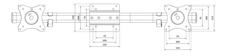
Neomounts Measuring unit: mm
